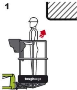
Machine and operator moving towards obstacle
