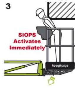
Machine stops Footswitch deactivated Manual override available
