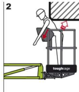
Operator pushed over the controls causing risk of sustained involuntary operation
